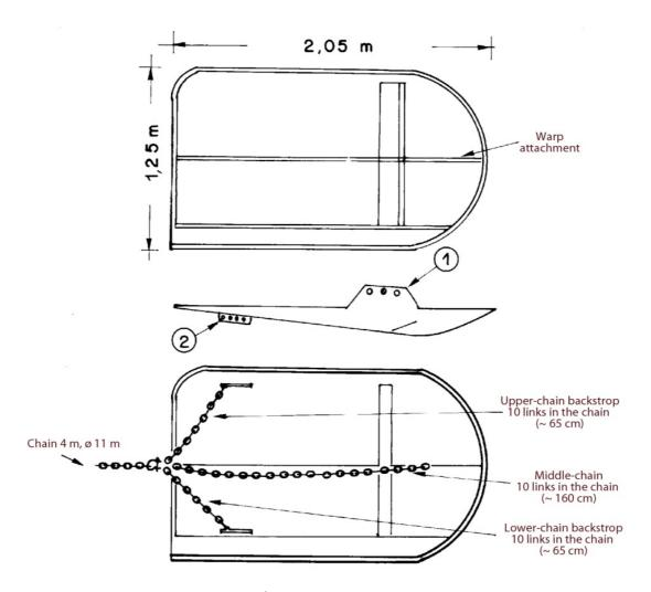
Fig. 6. Morgere WS8 (350 kg;  $2.5 \text{ m}^2$ ). The lengths of the backstrop chains are indicated without the shackles. The warp is shackled in the fore hole of the bracket sheet (see arrow 1). The short parts of the external crowfoot are shackled in the most back part of the backside sheets, upper and lower (see arrow 2).
