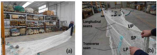
Figure XVI.1.9. Identification of the beginning and the end of each netting by looking at the transverse seams (a) and alignment of the transverse seams (b).
