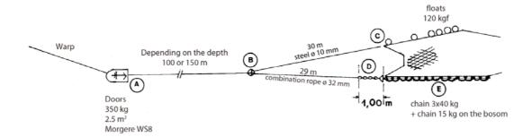
Fig. 3. Gear rigging details adopted for the MEDITS trawl. For the letter A, B, C, D and E refer to Figure 4.The length of the 1 m chain (D) must be adjusted in order to obtain the upper- (steel) and the lower-bridle (combination rope + chain) of the same length (30 m). See Figure 4 for further details.
