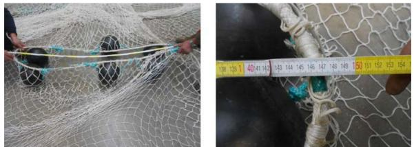
Figure XVI.1.4. Measurement of the headline at the bosom level. We measured 1.46 m, which multiplied by two is 2.92 m.
