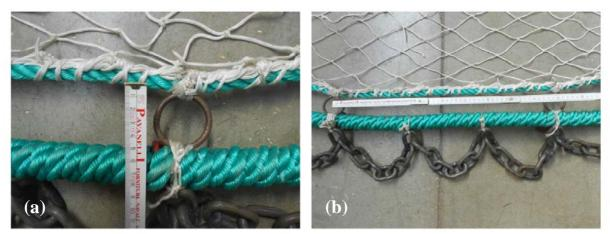
Figure XVI.1.2. In (a) measurement of the distance between the bolchline and the footrope (5 cm) and (b) between the bightings on the bolchline (50 cm).
