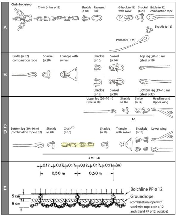
Fig. 4. Various details of the MEDITS trawl gear rigging. The length of the chain (\*) must be adjusted in order to obtain the upper- (steel) and the lower-bridle (combination rope + chain) of the same length (30 m). The ballast chain must be rigged at the tip of the lower-bridle.
